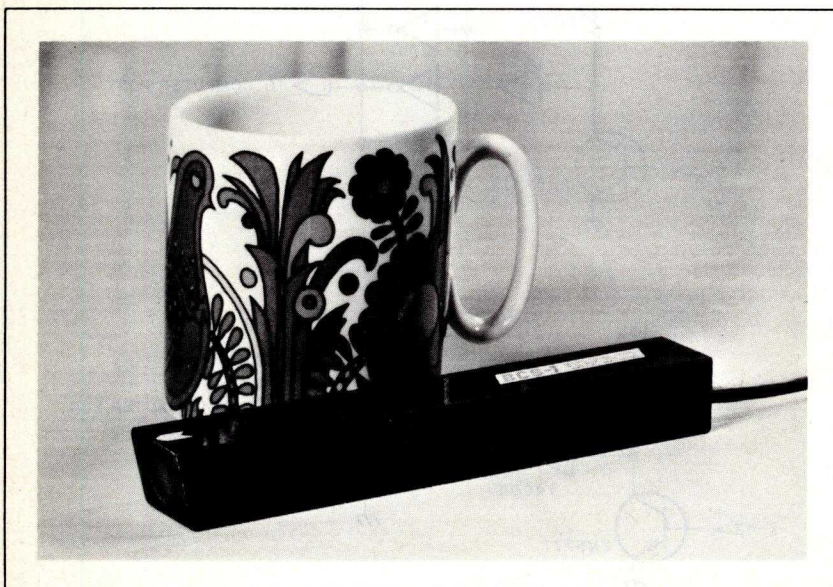
Photo 1: Micro-Scan Corp bar code scanner. Circular area at left contains aperture for viewing bar codes.
